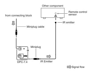
Only remote controller signals received by the DPC-7.4's IR IN are fed through to the IR OUT. Signals picked up by the DPC-7.4's remote control sensor are not output.
